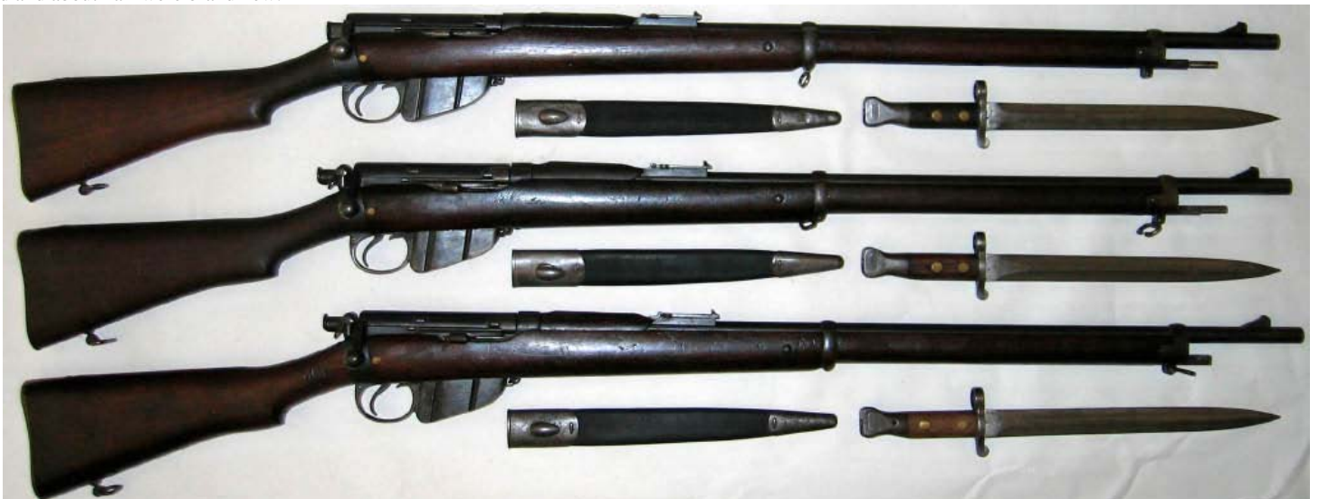
The three types of .303" donor rifles from the Boer War period. Top MLM MKII: Centre MLE MKI: Lower MLE MKI*
