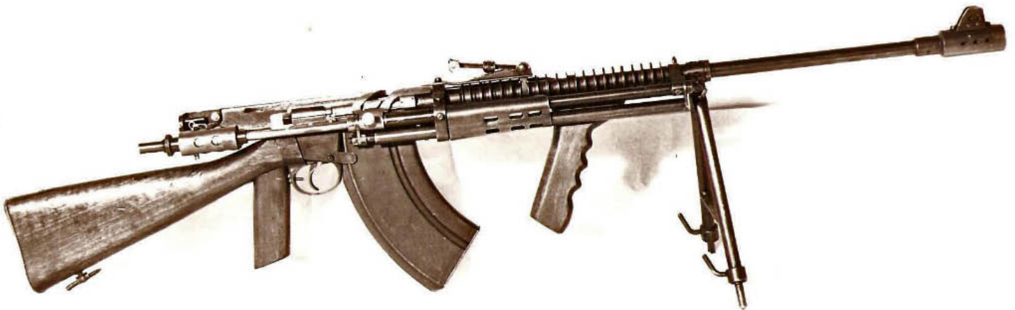
Right side of the completed Charlton Self Loading Rifle with its 30 round modified Bren Gun Magazine and bipod.
