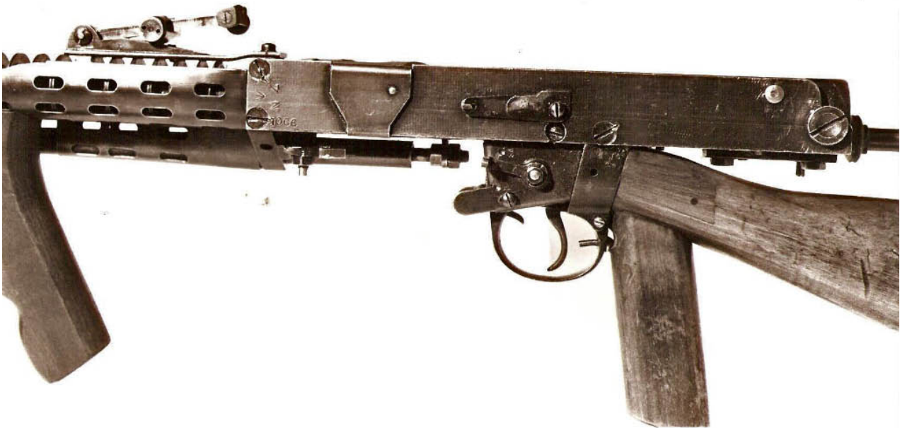
Left side of the completed Charlton Self Loading Rifle, Magazine removed. The receiver side plate is marked Broad Arrow NZ 1066.
