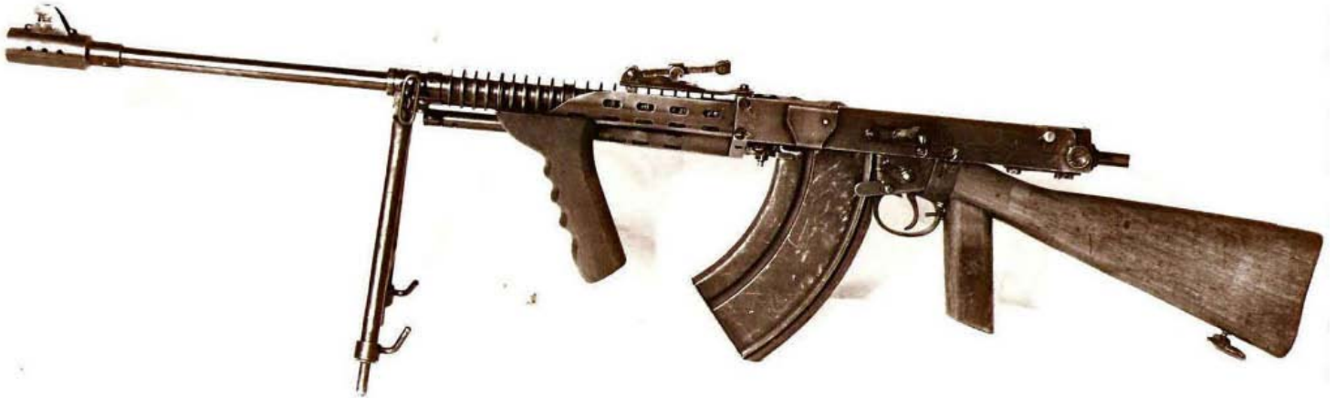
Left side of the completed Charlton Self Loading Rifle with its 30 round modified Bren Gun Magazine and adjustable bipod rest.
