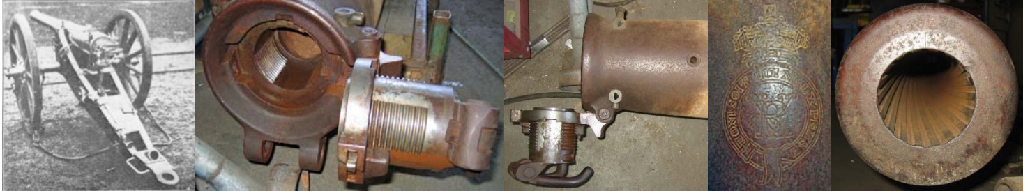
Left: MKI carriage with drag shoes fitted - connected by chains and cables to the wheel axle hubs and the trail. Second: Hinged breech screw assembly. Third: top view of breech and screw, vent – for friction match ignition - vent sleeve removed. Fourth: Queen Victoria monogram engraved on barrel denoting British Crown / Government ownership. Right: Muzzle showing rifling and Barrel Serial Number
