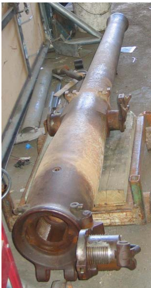
Left: MKI 15pdr barrel breech open, showing front and rear gunsight mounting blocks, breech vent, and trunnions Right: New Zealand gunners in action with their Breech Loading 15pdrs on MKI carriages, a two gun Battery in the Boer War c1901.
