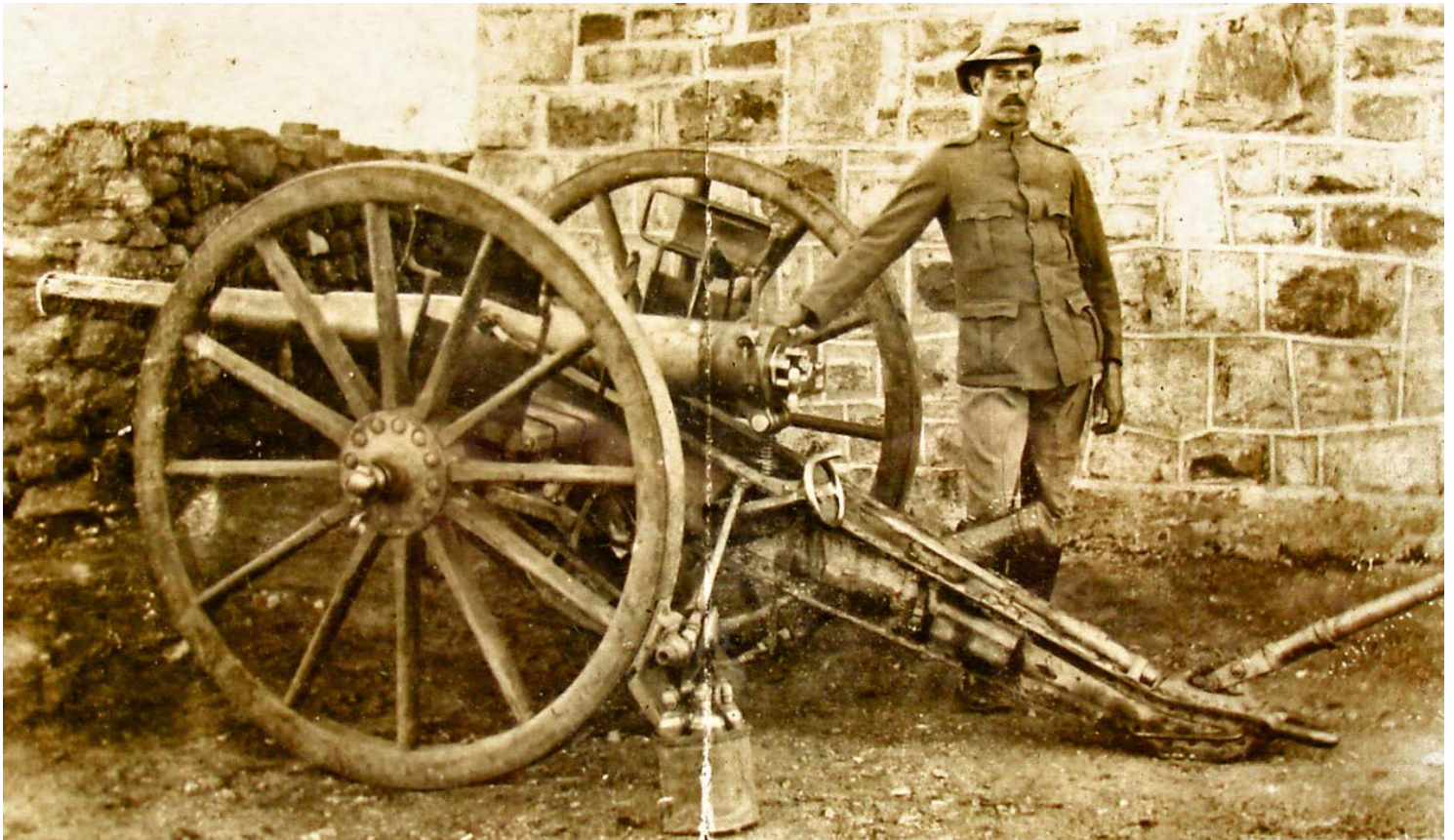
W Taylor New Zealand Mounted Rifleman c1900 at the Blockhouse on the Kopje overlooking the town of Brandfort. Courtesy Noel Taylor 15pdr BL barrel mounted on a MKIII or MKI* or MKII* converted carriage. Note the "spade" beneath the trail which dug in when the gun recoiled, connected by a rod to a compression spring in the cylinder on the trail allowing the gun to recoil and then be returned to its original firing position.
