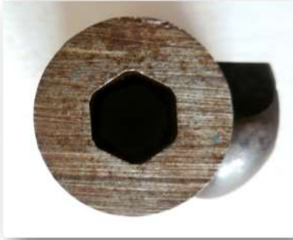
Cross-section of a Whitworth barrel illustrating the hexagonal bore
