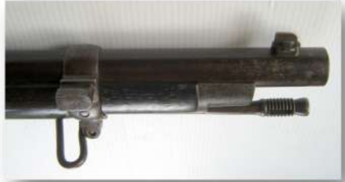
Foresight, bayonet bar and ramrod of Whitworth Short Rifle
