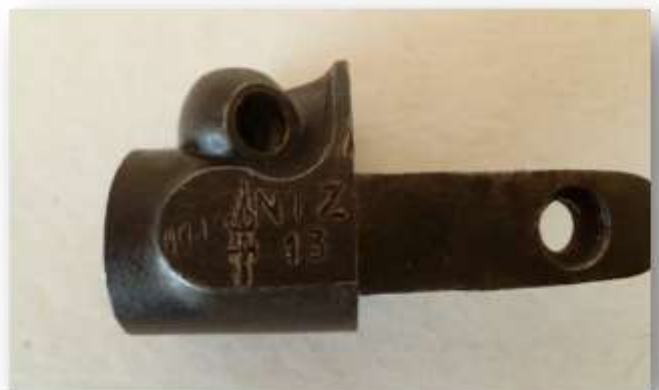
Breach plug end section of Whitworth rifle serial No D 430. It also is N^Z 13 marked, forward of this it is stamped No.16 which over stamped with a cancelation (of number) mark. This is a section of a cut up New Zealand Army disposed Whitworth.
