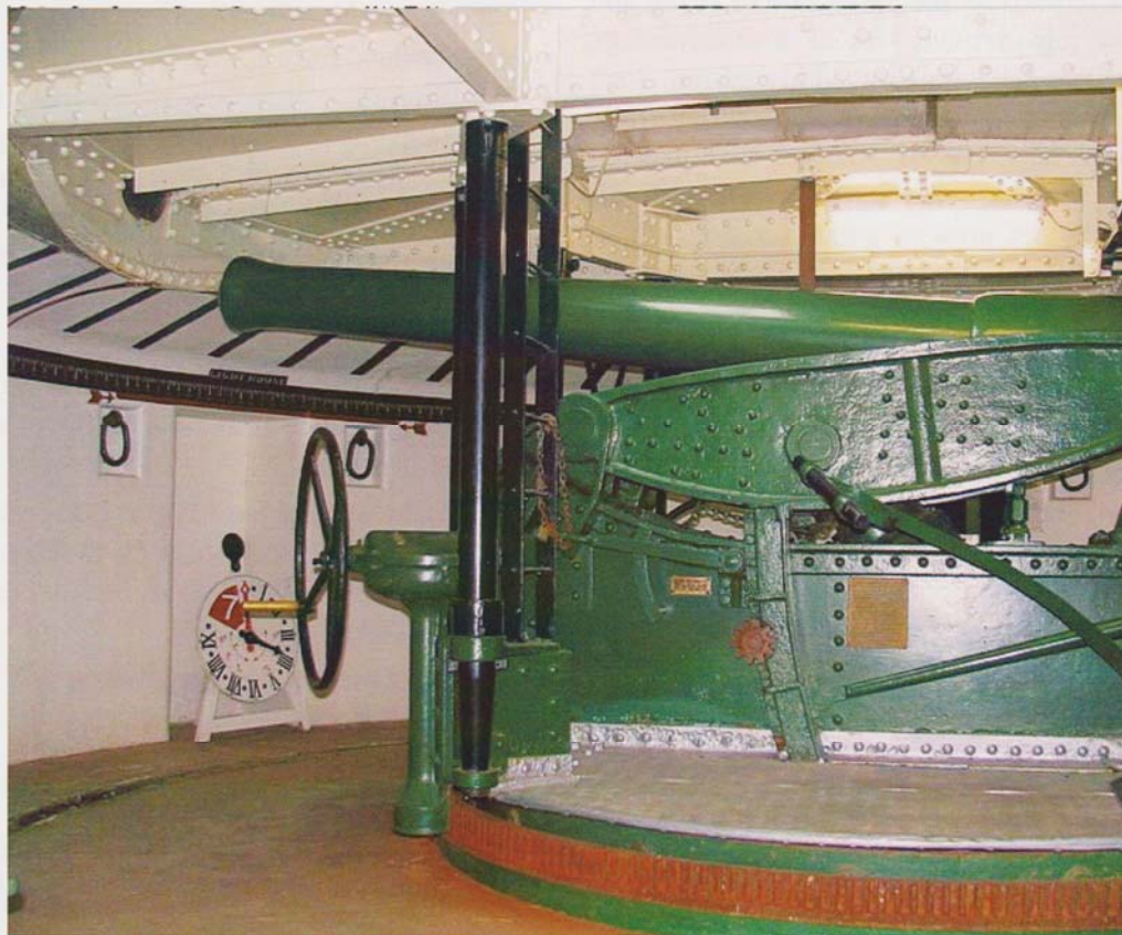
Armstrong BL 6-inch Mk V Disappearing Gun at Tairaroa Head, New Zealand
