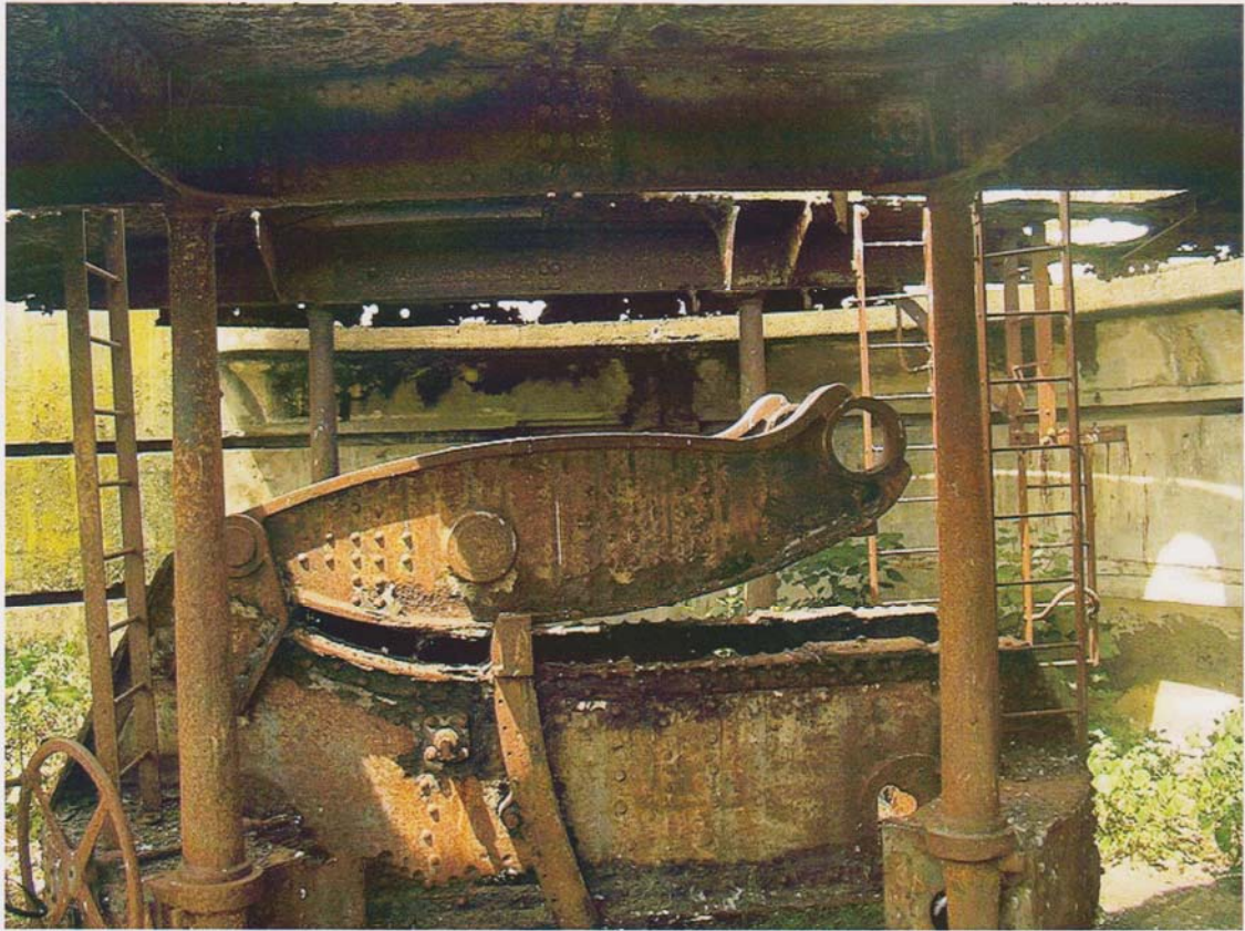
The mount for an 8-inch (200 mm) Disappearing Gun at South Channel Fort Victoria showing the hinged retraction mechanism, Victoria
