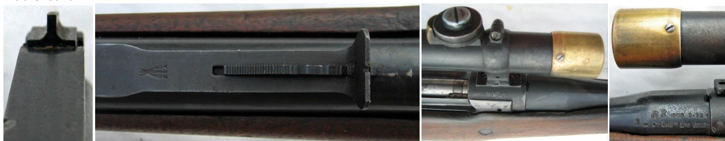
BSA P14 sporter blade foresight dovetailed for windage adjustment, U rear sight. BSA Serial No M 9124. Proof marks for 41grs Cordite & 215gr Bullet.
