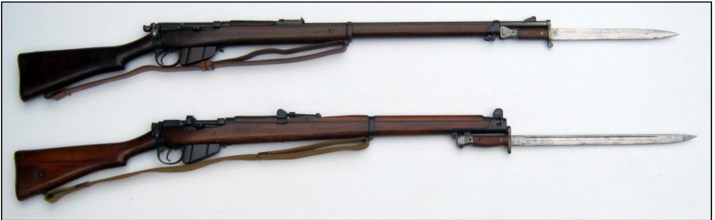
Top: Magazine Lee Enfield Mk I* and Pat. 1888 Bayonet sighted for Mk VI .303 cartridge. Used by NZ Infantry. Bottom: Short Magazine Lee Enfield Mk III and Pat 1907 Bayonet sighted for Mk VI .303 cartridge for NZ Forces and Mk VII cartridge for Australian Forces. Used by NZ Mounted Rifle, Artillery and Engineers and all Australian Forces.
