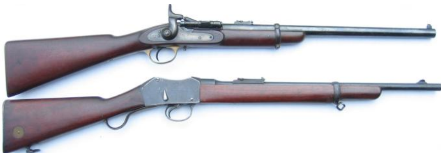
Top: .577 Snider Carbine cut down from a rifle
