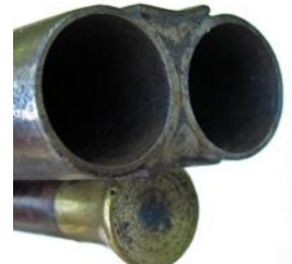
Musket bore 29" barrel hooked breech smooth bored percussion Tupara (double barreled musket) the Maori warriors favorite firearm, fired the older standard British military ball cartridge sometimes both barrels together also buck shot etc, very effective at close range.
