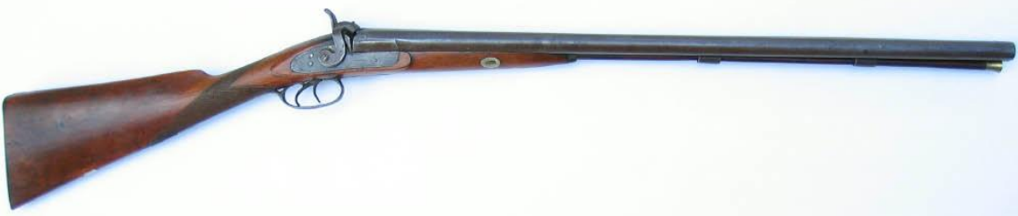
Musket bore 29" barrel hooked breech smooth bored percussion Tupara (double barreled musket) the Maori warriors favorite firearm, fired the older standard British military ball cartridge sometimes both barrels together also buck shot etc, very effective at close range.
