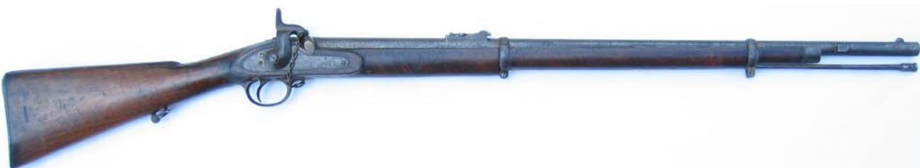
25 bore (.577" caliber) 33" barrel Enfield short Rifle pattern 1856 and later variations all with iron furniture for land service sergeants together with a Yataghan sword bayonet below. A similar short Rifle pattern 1858 with five groove rifling and brass furniture for sea service together with a pattern 1859 cutlass sword bayonet image below carried in a black leather scabbard.
