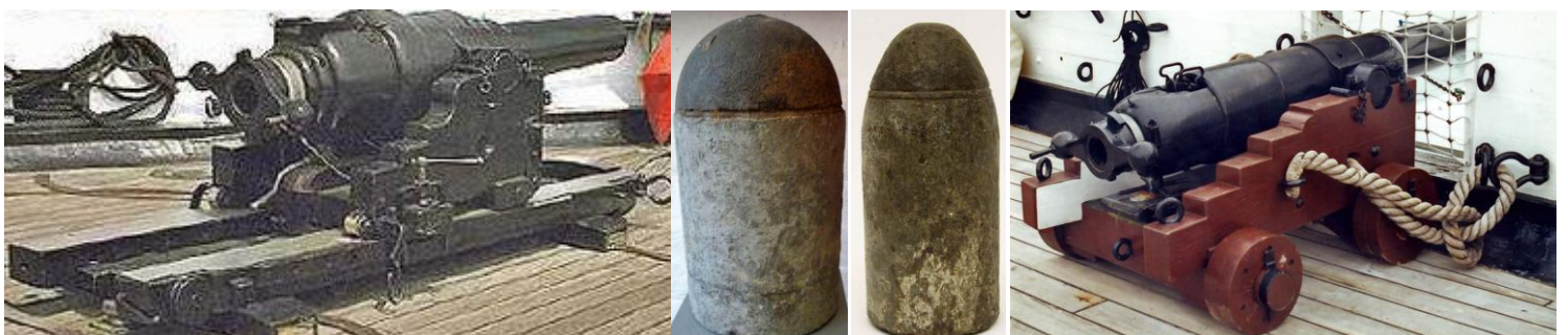
Left: 110 pounder 7" caliber Rifled Breech Loading Armstrong gun shown mounted on a sea service sliding carriage on the upper deck as a bow chaser which could be slewed across the deck on heavy brass rails, recoil checked by the breeching ropes. Centre: lead coated shells for the 110pounder 7" and 40pdr 4.75" Armstrong. Right: a 40pounder 4.75" calibre Armstrong RBL gun mounted on a trucked (wheeled) sea service carriage. Types used at Gate Pa
