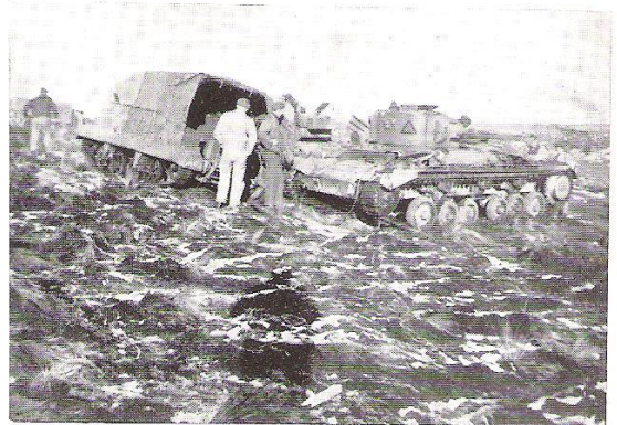
THE SLAVE BATTERY CARRIER GIVES A TANK ITS FIRST START IN THE MORNING.
