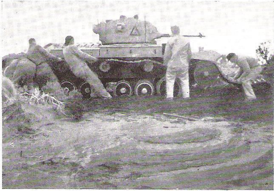
REPAIRING A TRACK BROKEN IN HEAVY SAND.
