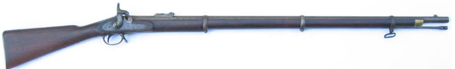
25 bore (.577" caliber) 39" barrel Enfield Long Rifle pattern 1853 together with a triangular 17" blade socket bayonet carried in a black leather brass capped scabbard. Locking ring on socket
