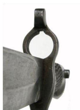
the stabilizer notch in the muzzle ring
