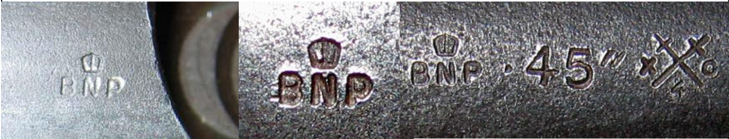
British proof on bolt to rear of finger cocking hole. roof mark on receiver body.
