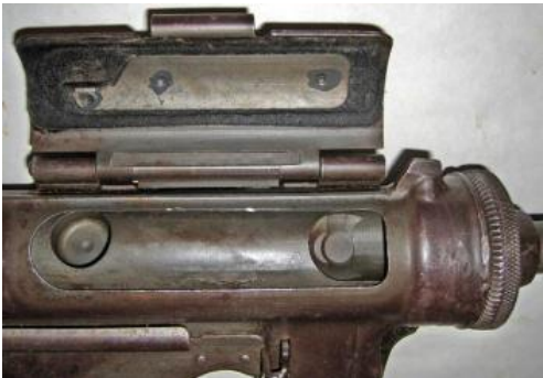
British proof on bolt to rear of finger cocking hole. roof mark on receiver body.
