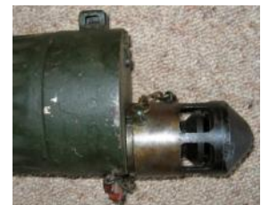
Muzzle attachment, foresight & hose connection, drain plug
