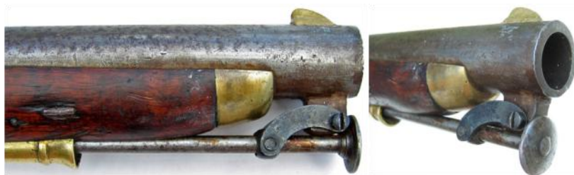
Saddle bar and ring, rear sight, Birmingham private proof marks Lock marked TOWER / PROOF & Crown
