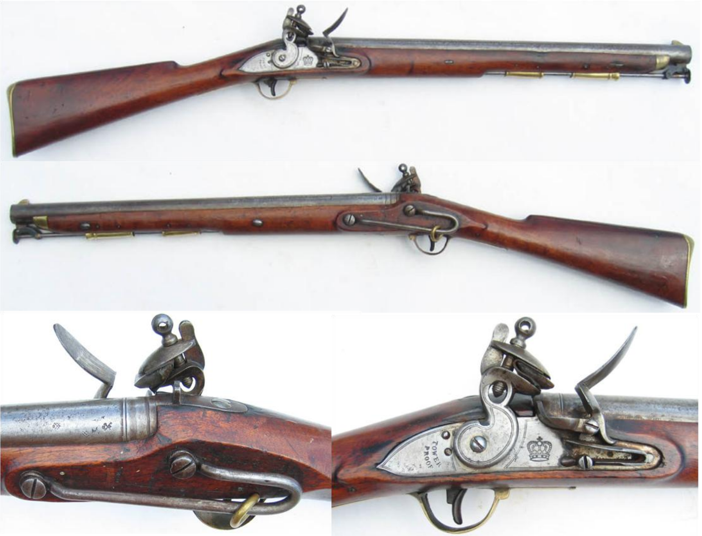
Saddle bar and ring, rear sight, Birmingham private proof marks Lock marked TOWER / PROOF & Crown
