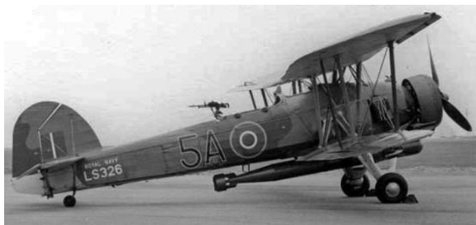
Fairey Swordfish showing the rear mounted Vickers GO "K"
