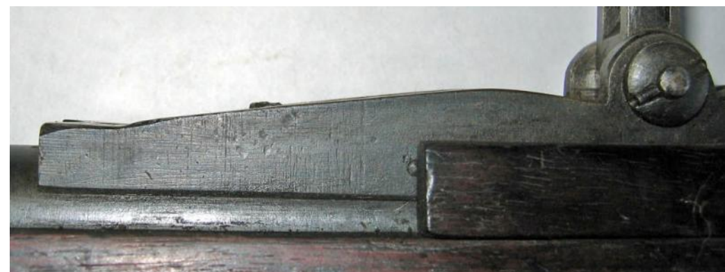
Above: ShtLE rear sight ramp for MKI***HV, MKIIIHV to suit MKVII HV ammunition - 174gr projectile.
