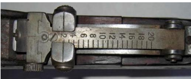
Rear sight leaf graduations for ShtLE MKI left & MKI*** right which are the same.
