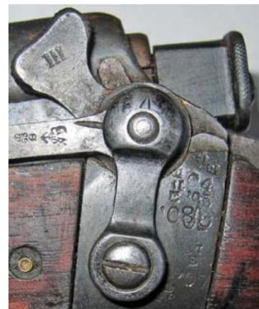
Barrel & receiver marks on 1903 MKI. showing conversion to MKI* in 1905, to MKI** in 1908 and MKI***HV in
