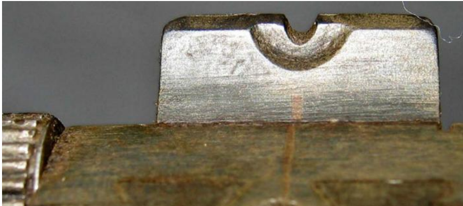
Rear U sight fitted to ShtLE MKI** MKI*** & MKIII with windage adjuster. Front Blade sight fitted to MKI**, MKI*** & MK III
