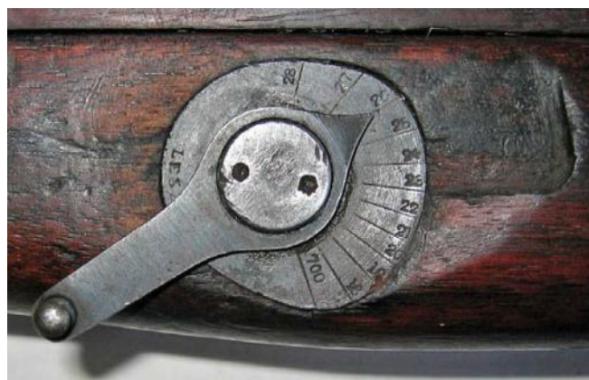
Left: Front long range dial sight for MKI, MKI*, MKI** & MKIII to suit MKIIC to MKVI ammo - 215gr projectile. Right: Front long range dial sight for MKI***HV & MKIIIHV to suit MKVII high velocity ammo - 174gr projectile.
