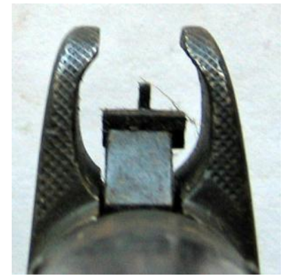
Rear U sight fitted to ShtLE MKI** MKI*** & MKIII with windage adjuster. Front Blade sight fitted to MKI**, MKI*** & MK III
