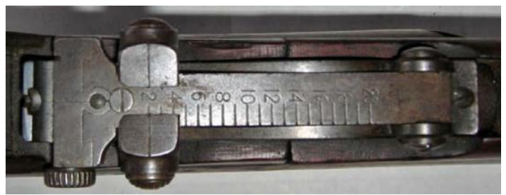
Rear sight leaf graduations for ShtLE MKI left & MKI*** right which are the same.
