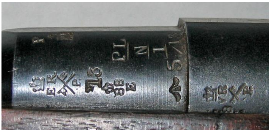
Barrel & receiver marks on 1903 MKI. showing conversion to MKI* in 1905, to MKI** in 1908 and MKI***HV in
