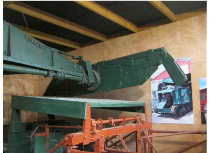
Universal (Bren gun) Carrier converted to hedge trimmer
