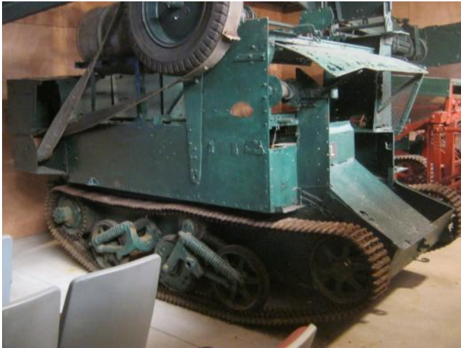
Universal (Bren gun) Carrier converted to hedge trimmer
