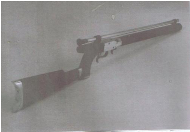
Brian Redwoods personal Buggy Rifle. Under Hammer target pistol-carbine 14 inch octagonal barrel in .40 calibre 1 1/2" across the flats with saw handle type pistol stock with a detachable shoulder stock
