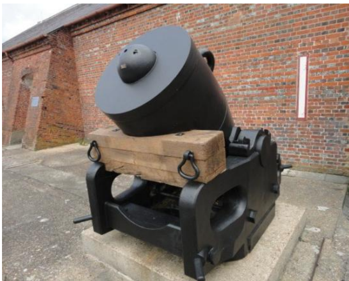
113" 1856 Mortar & Bed. This beast was donated by the Royal Armouries in 2000 having come from one the Portsmouth Hill Forts. Manufactured 1856 by FP & Co, this was capable of firing 2.8 km a 90kg filled shell. Weight - 3,500 kg ?
