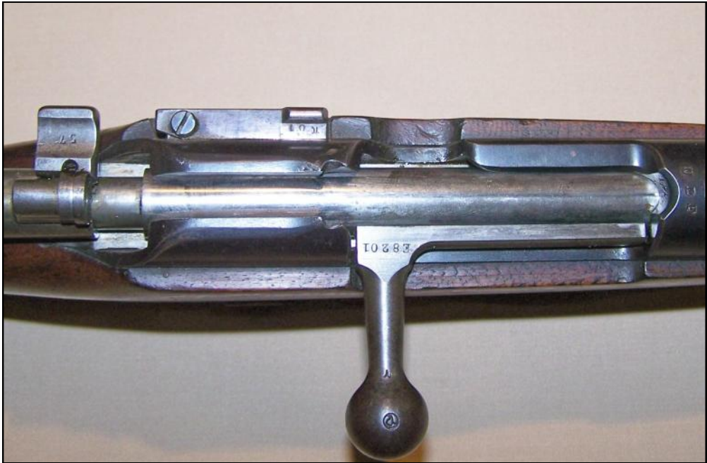
M 1904 Action. Note the split receiver bridge and bolt handle base which serves as an emergency locking lug.
