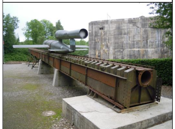
Hazebrouck - The V1 rocket mounted on a portion of original ramp. Here, the tube in which the piston was fired can clearly be seen. The piston had a lug project-
