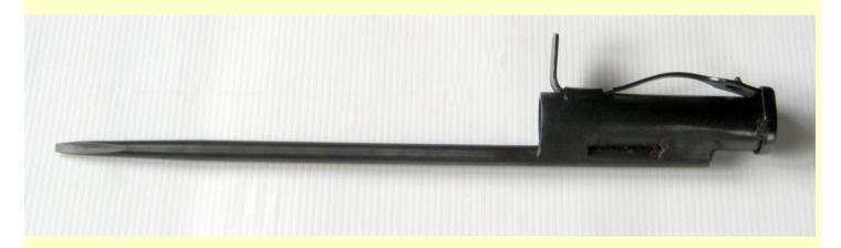
Approved on 23 September 1942 the Sten Machine Carbine Bayonet Mk I was designed to be used with the Mk II Sten. It comprises of an 10.8 inch (274 mm) spike welded to an 3.8 in (96 mm) socket with a sheet steel end cap and internal diameter of 17.5 mm, a bent leaf spring sits on top, which engaged in the barrel shroud of the sten. The No 4 scabbard was used with this bayonet.
