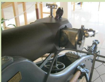
Detail of breech, the new block was machined from a solid block of steel
