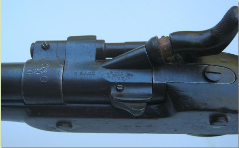
Mk III breech block Snider Patent acknowledged
