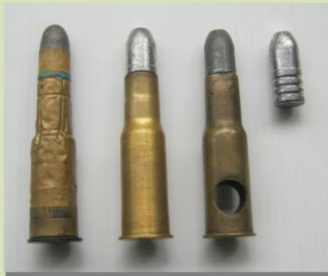
Ammo: foil, drawn brass, dummy, projectile
