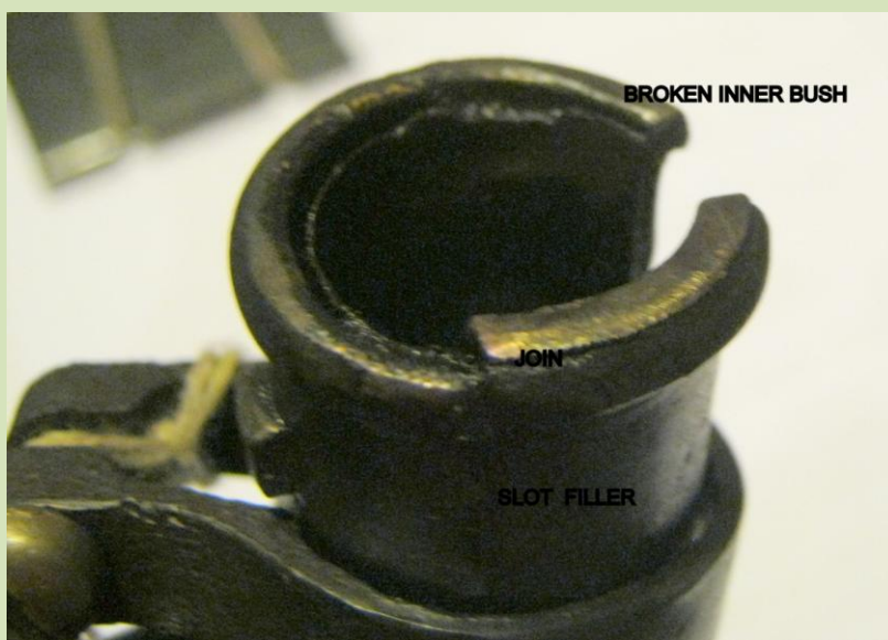
A broken socket, note how thin the bush is
