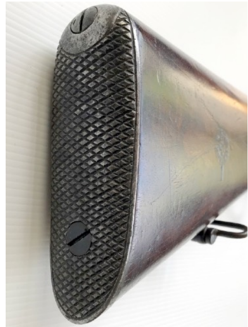
Both the chequered butt plate and sling swivel were dropped from the final third pattern
