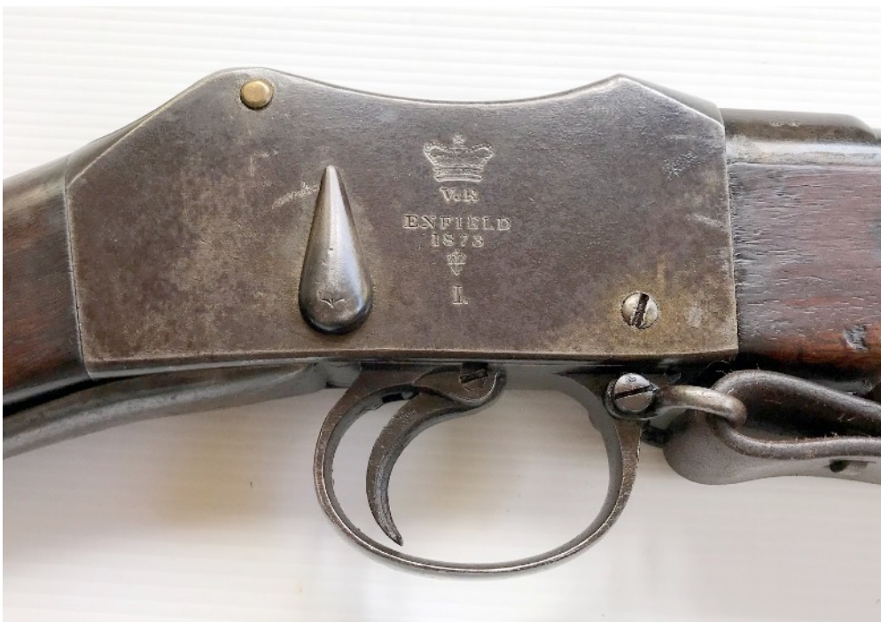
Second pattern action body Note bronze axis pin and early type trigger group.
