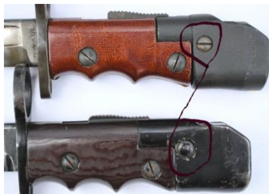
The socket locking pin is a bolt, not a slot head screw.
