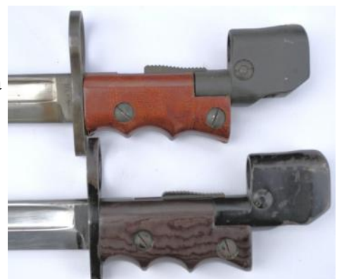
The socket locking pin is a bolt, not a slot head screw.
