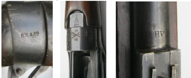
Typical marking found on MLE upgraded with BSA commercial barrel & action
