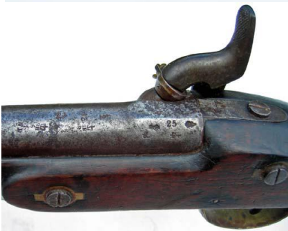
Private London proof marks & 25 bore plus Ordnance proof & acceptance marks on barrel.
