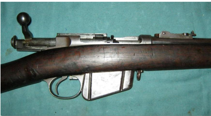
M 1885 Lee bolt action and detachable magazine, this version of magazine designed by L P Diss
