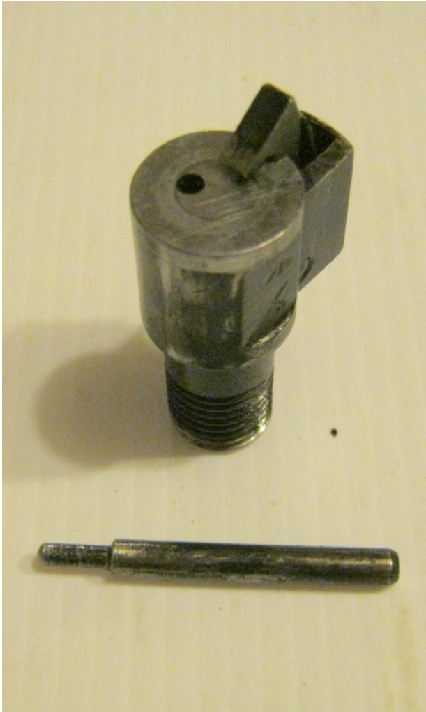
Modified bolt head & firing pin
