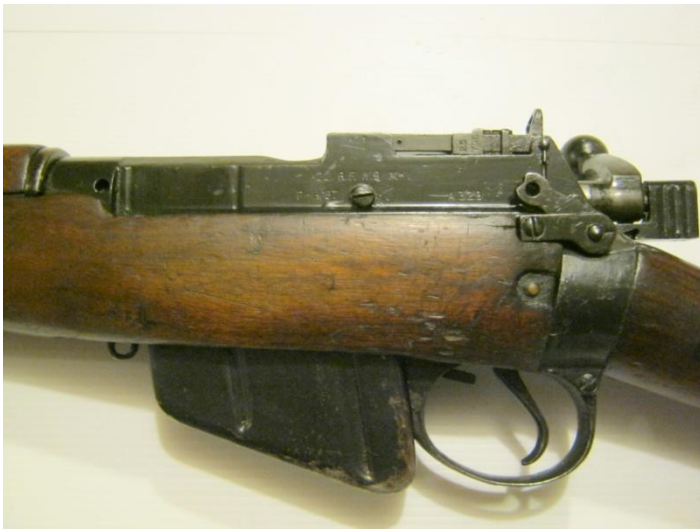
LHS of receiver wall marked: .22 RF N 9 Mk I P-H '57 A329
