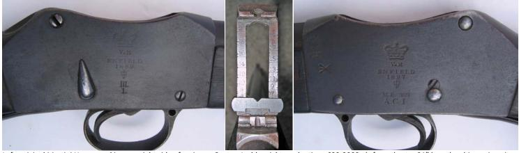
Left; original Martini Henry markings on right side of reciever. Centre; Ladder sight graduations 600-2000yds for a shorter 21" barrel carbine using nitro powder (cordite) Right; Martini Enfield conversion markings on left side of carbine reciever fitted with a 21" barrel with Enfield 5 groove rifling, diameter of bore .303", depth of rifling .0065", width of lands .0936", twist 1 turn in 10" left hand. >< sold out of British Service
