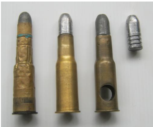
Ammo: foil, drawn brass, dummy, projectile
