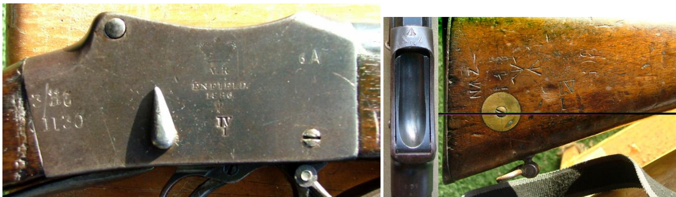
NZ Issued Martini Henry Mk IV No 471, short lever, showing 1890 issue marks and also Home Guard service in WW II
