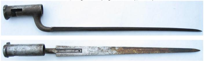
Top view showing slot for spring catch, which is missing in this example.
