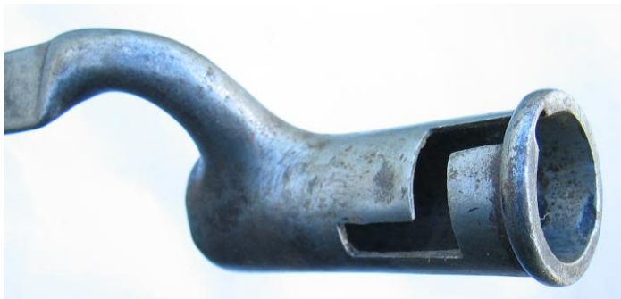
Socket showing 3 motion slot and collar for Hanoverian catch.
