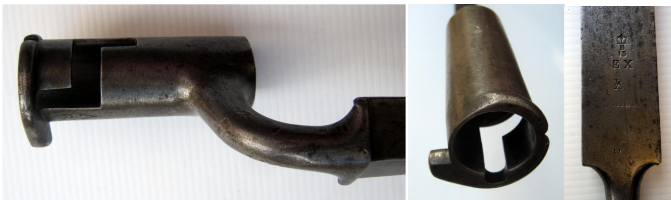
Left and centre: Socket showing Lovell lug, note notch to reveal foresight.
