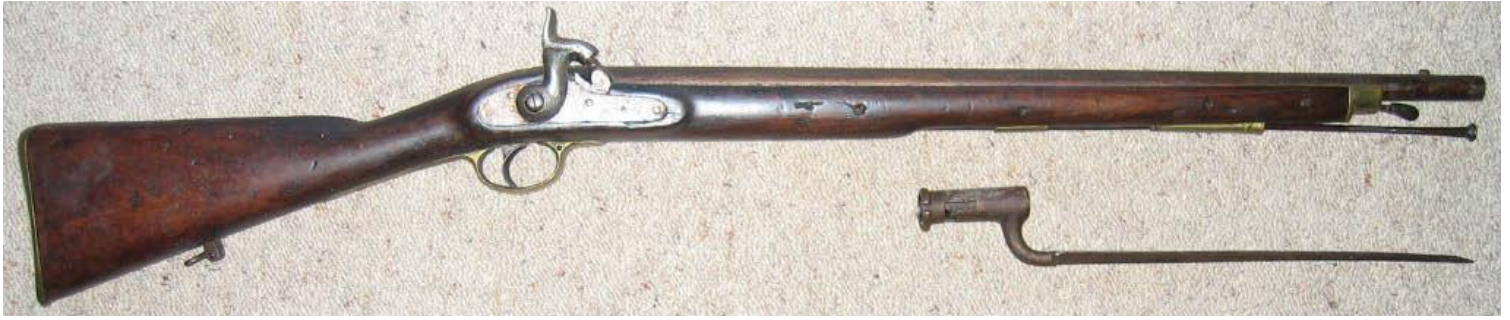
Lovell's 26" barrel Pattern 1840 17 bore (.653" calibre) constabulary percussion carbine with its 13" triangular blade bayonet 3" socket
