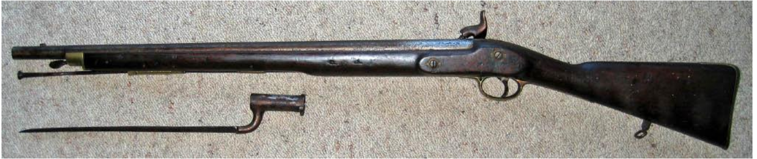
Barrel pined to walnut stock, brass furniture including two ramrod pipes, fore end, trigger guard and buttplate.
