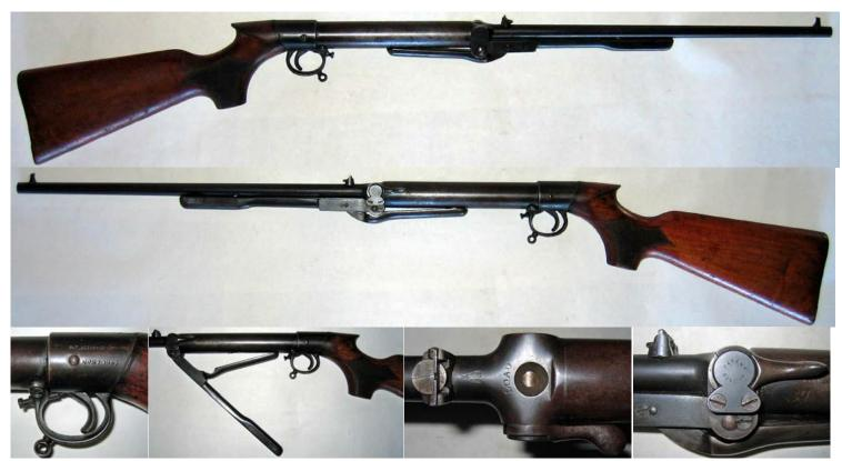
Left image: trigger adjustment using a threaded screw through the trigger guard. Second: cocking under lever with side-catch release. Third: Rear sight screw elevator calibrated for 10, 15, 25 and 50 yards. Right: Loading lever is moved upwards & the lead pellet droped in.
