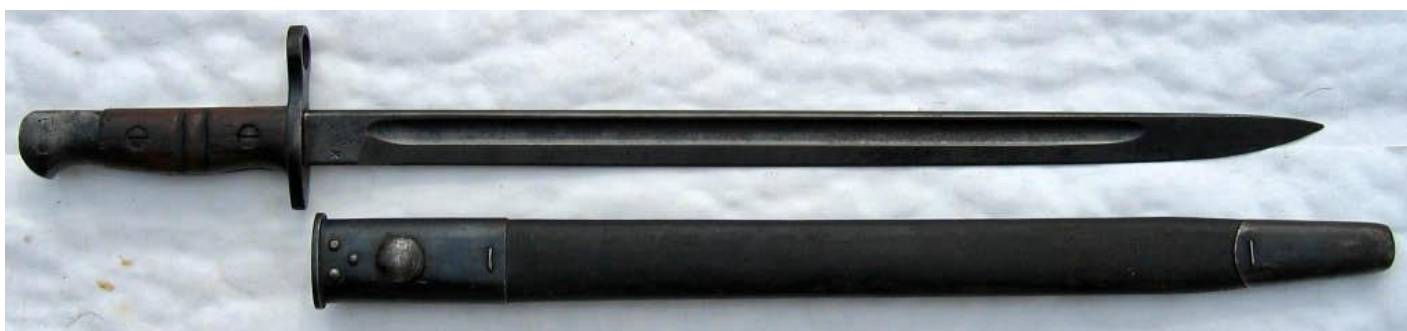
Pattern 1913 bayonet for P 14 Rifle, made by Winchester, Also made by Remington and Vickers, Note two gooves in the grips to distinguish it from the Pat 1907.
