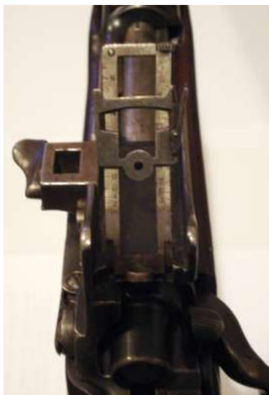
Winchester fine adjustment rear sight
