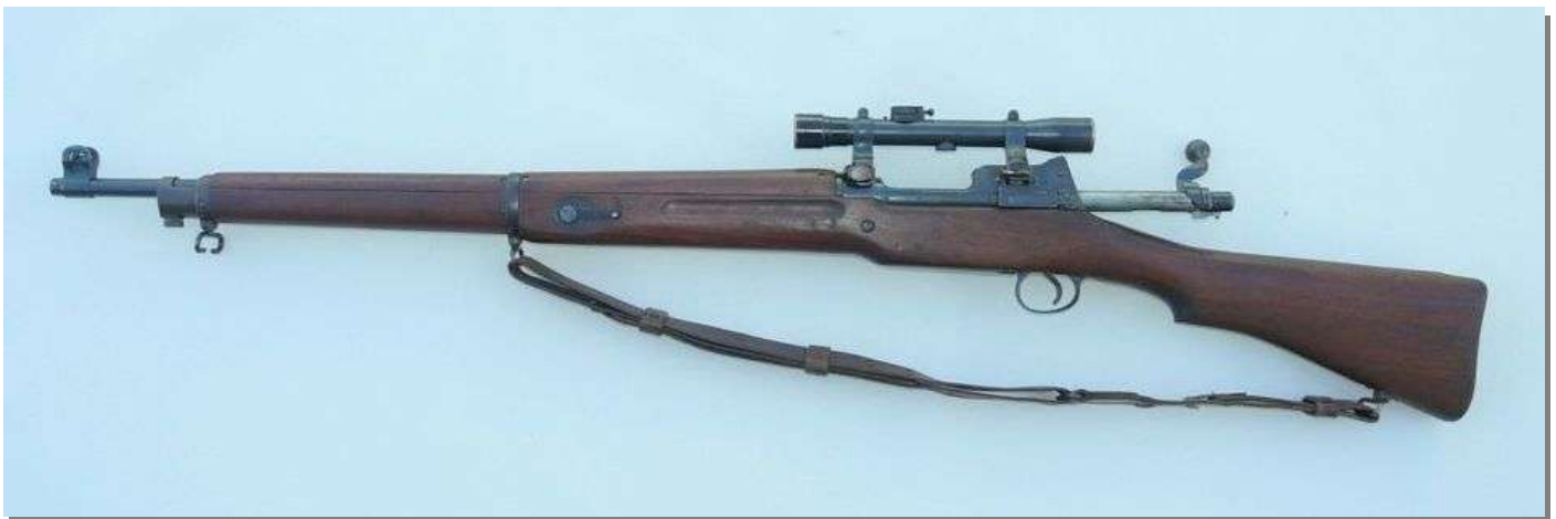
Right and left views of P 14 Mk I* (T) made by Winchester with Pat 18 telescopic sight by Periscope Prism Co.
