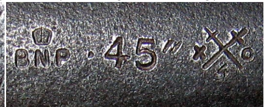
British proof marks on barrel
