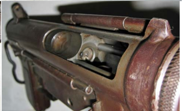
Ejection port cover open showing bolt back in firing position
