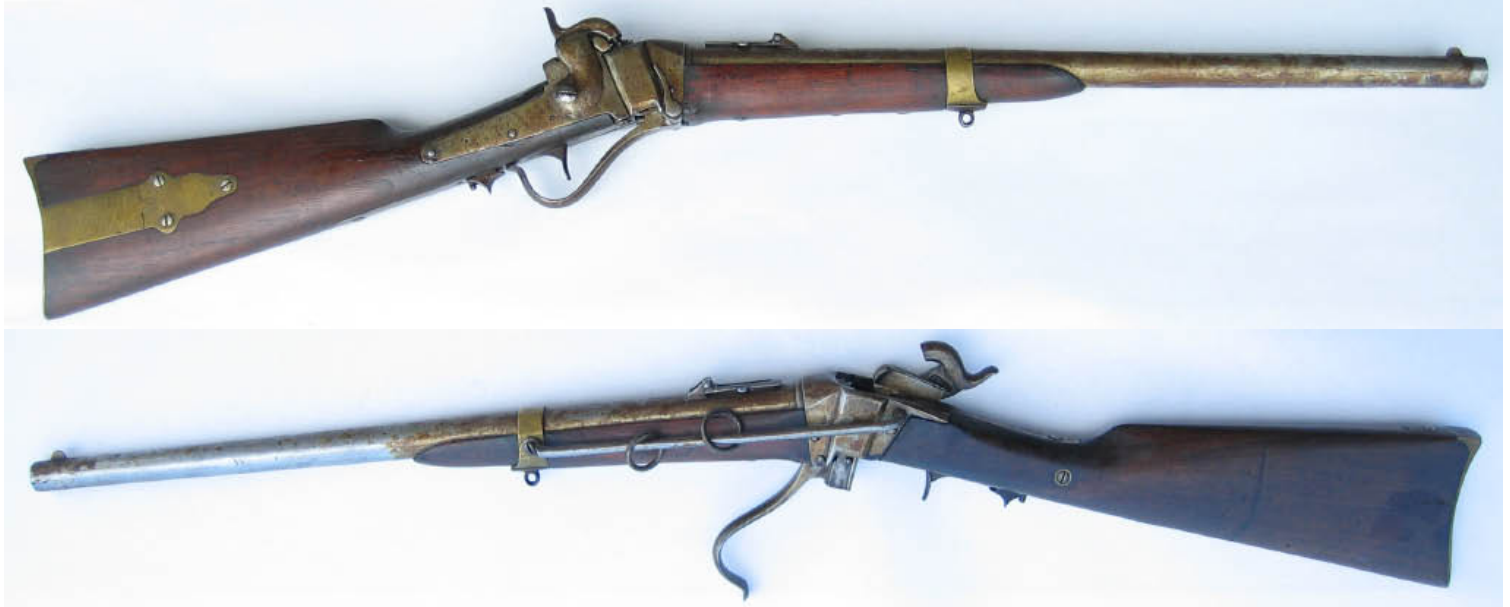
Left side showing saddle bar and two rings. Loading lever down which lowers breech block and exposes chamber for loading.
