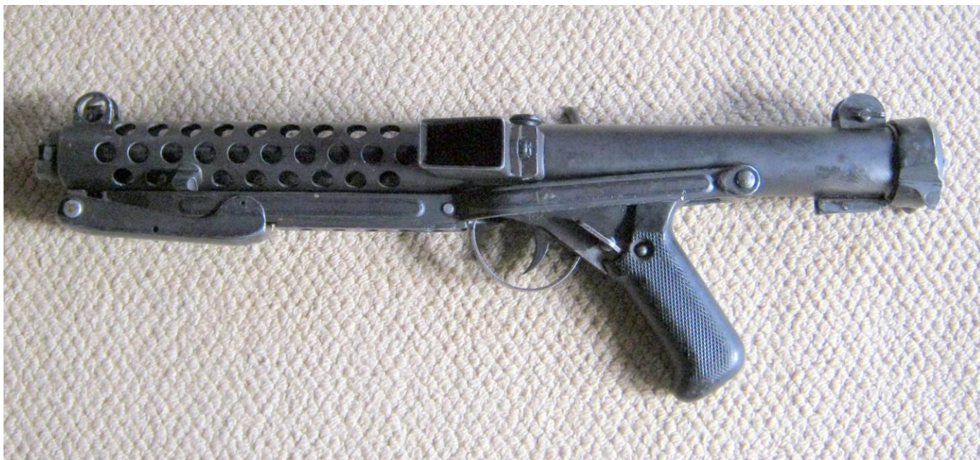
Sterling Mk II No KR 2725 with butt folded, embodies many of the MK III features.
