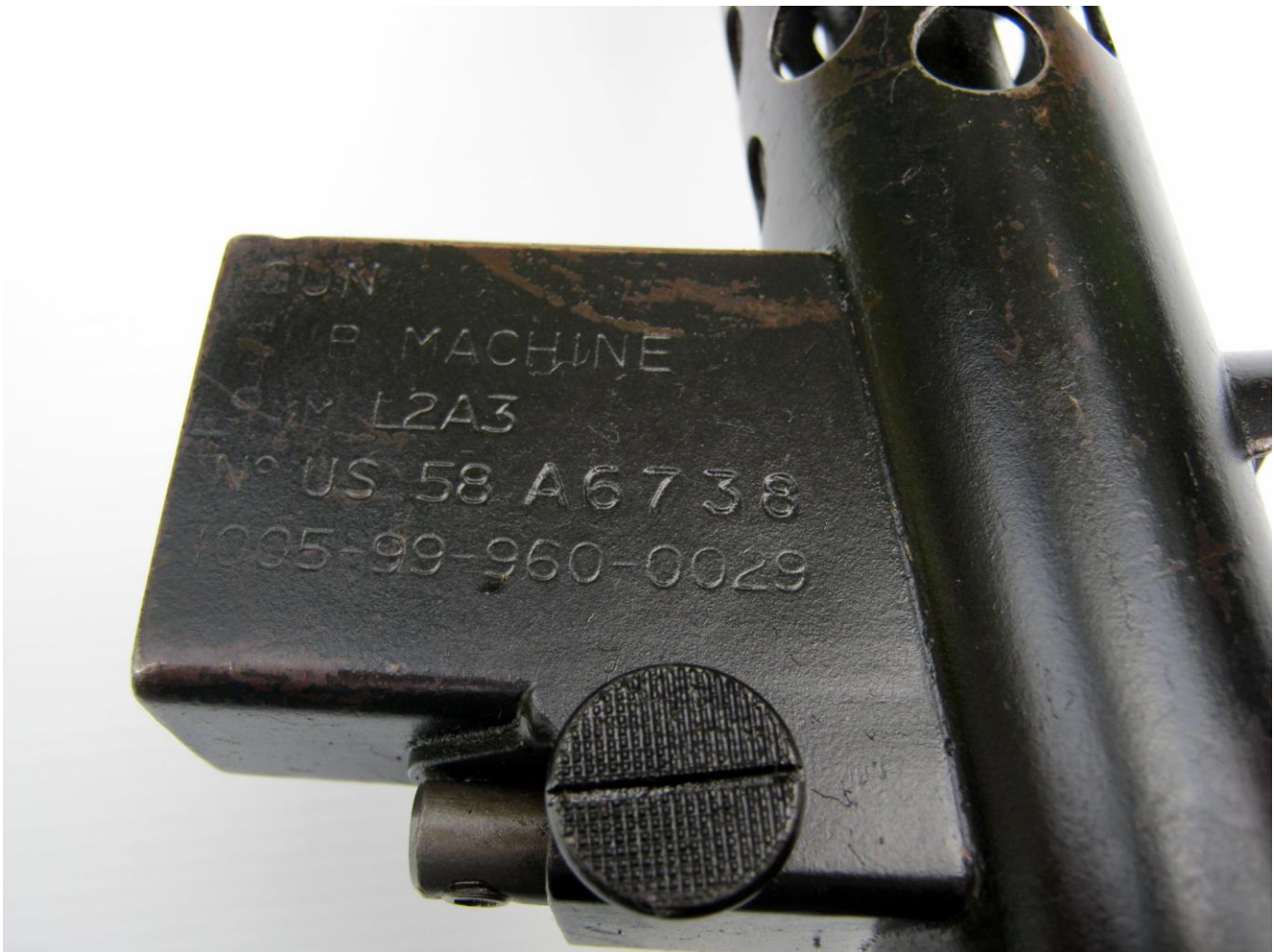
Marking on Sterling manufactured Mk 4 L2A3, Fazakerley manufactured guns have serial prefix UF
