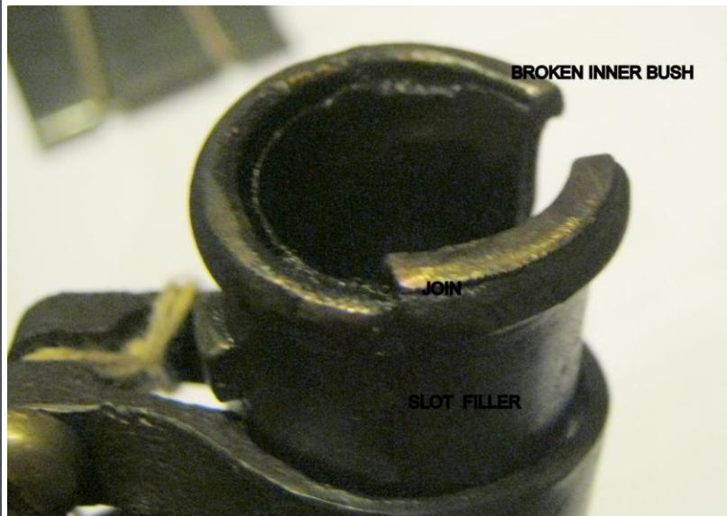
A broken socket
