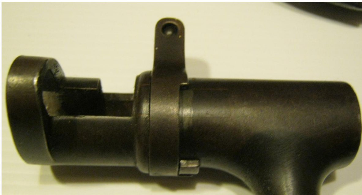
The filled section of the original slot can be seen in front of the locking ring in line with the new slot.
