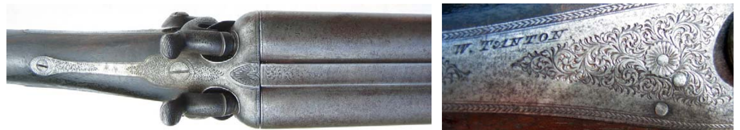
Left; Topside of engraved steel action & tang, firing pins could be replaced with percussion nipples & the gun muzzle loaded with musket ball cartridges Right; Engraving on right side back action lock plate .
