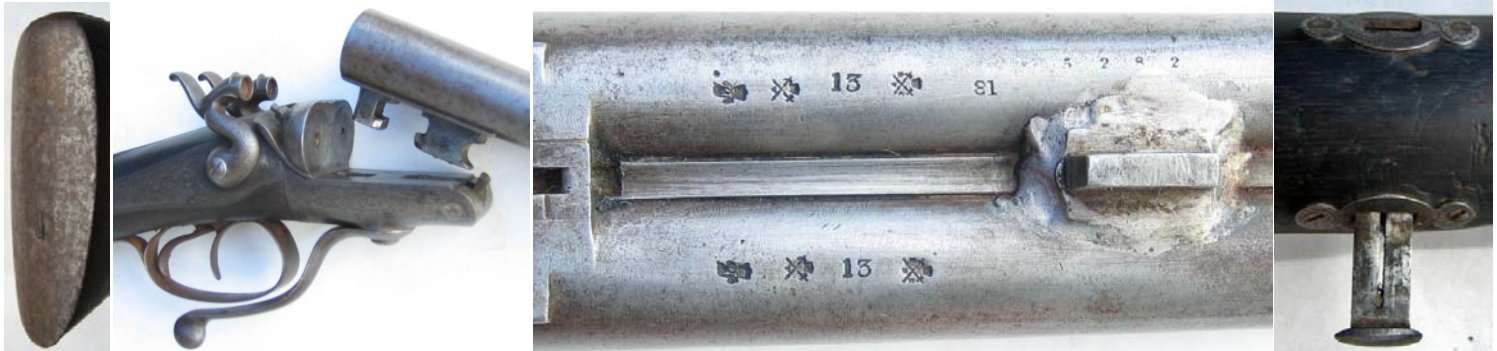
Plain steel butt plate. Under lever action showing locking design. Birmingham private proof marks and Gun serial No 5282. Fore end locking wedge
