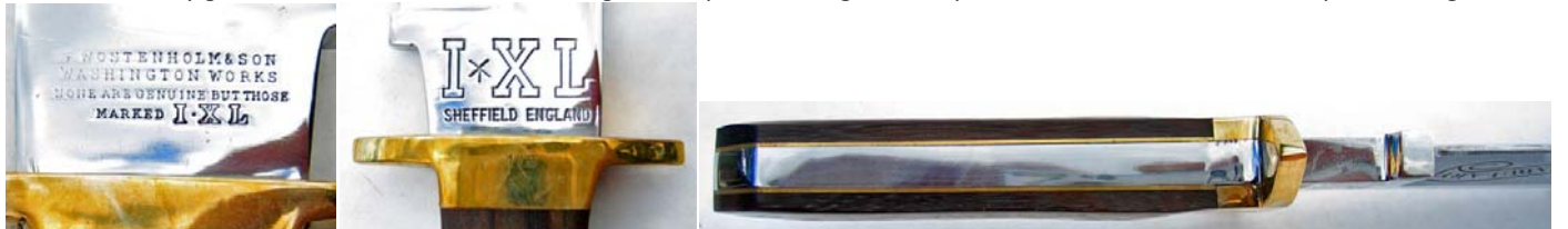
Marked G. Wostenholm & Son / Washington Works / None Are Genuine But Those / Marked I*XL. Brass shimmed between carbon steel tang and rosewood grips.
