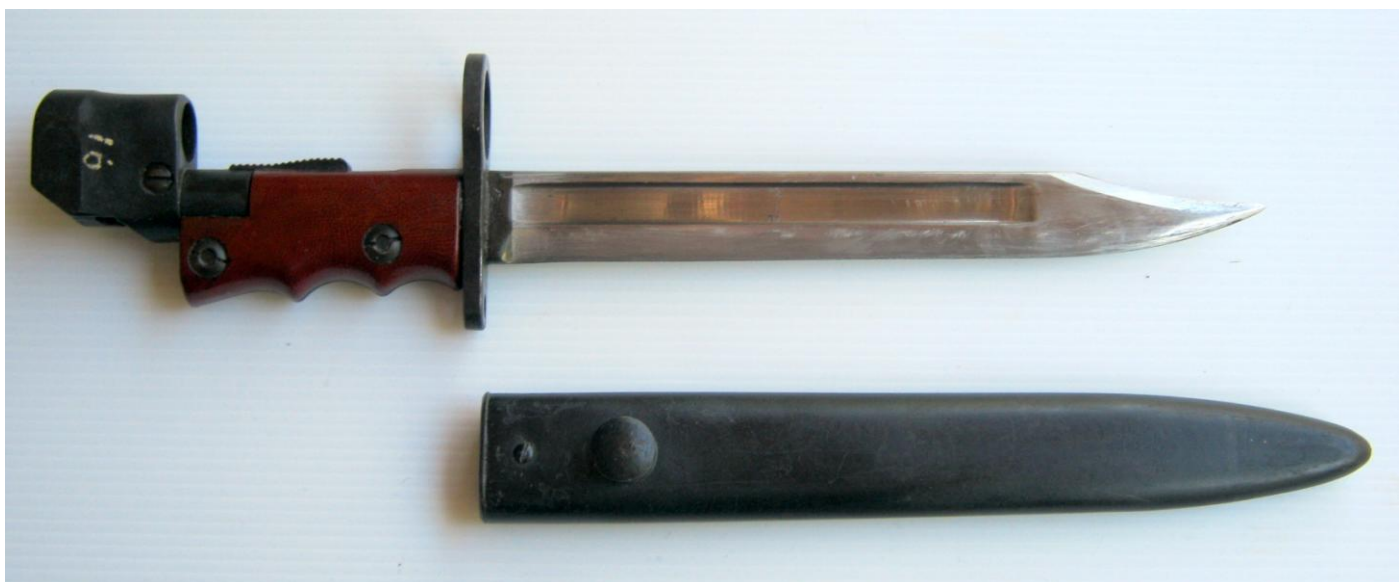
No 7 Mk I Bayonet & scabbard, the socket rotates to form a fighting knife. Developed in 1945 for the MK V Sten it was also used on the No 4 Rifle. Manufactured by Elkington, ROF Poole, ROF Newport and BSA. 330,000 made.
