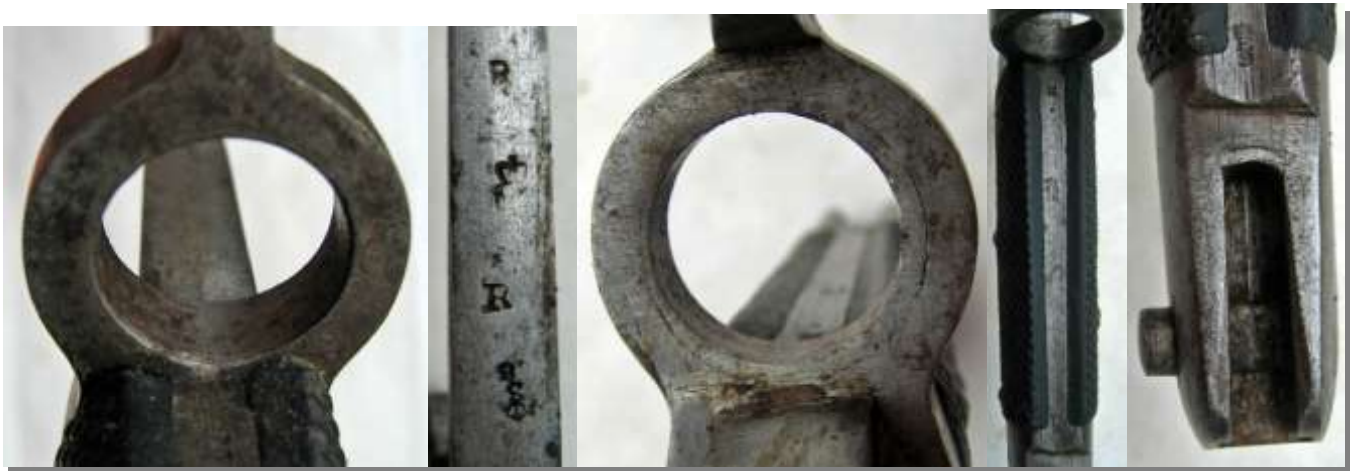
Yataghan bayonet Pattern 1860 (converted in February 1885) to fit Martini Henry Rifle. Note bushing and filed step to the hilt
