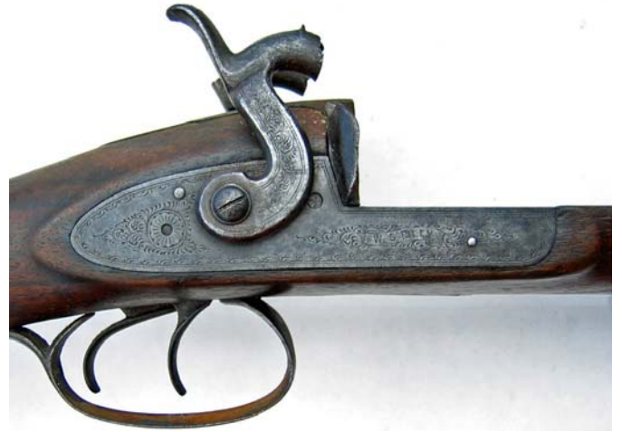
Hammer on half cock. Side locks easily removed for servicing.
