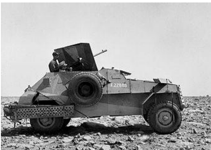
Mk II fitted with Breda gun
