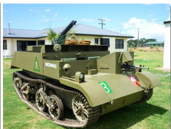
Later Carrier LP 2 welded construction
