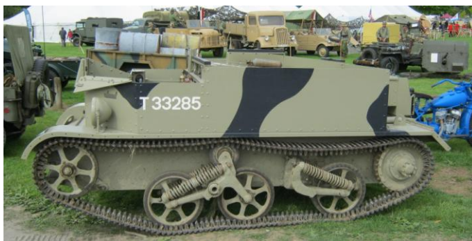
Early Carrier Bren LP No 1 (NZ) riveted construction
